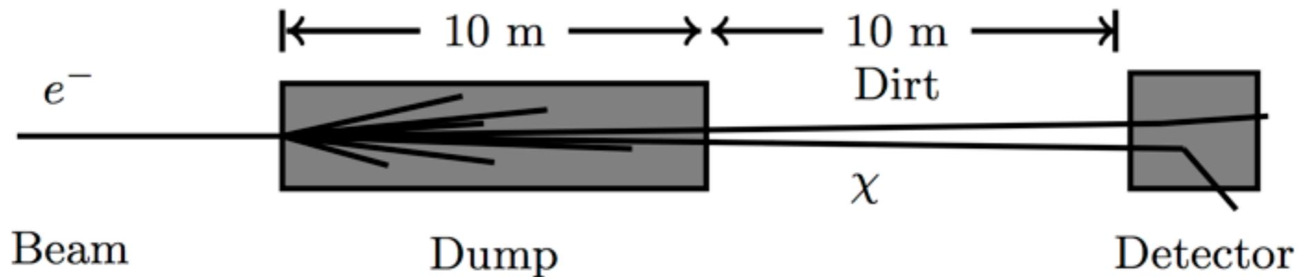
Aluminum dump, 12 GeV beam (pulsed)
