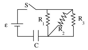
**Answer:** Note that the resistors are all in parallel. So the equivalent resistance  $R_{eq}$  is given by
