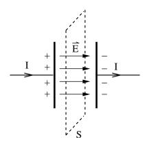
Let's calculate  $I_d$  for a parallel plate capacitor where the plates each have area A. Then the flux through a surface S between the plates is
