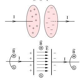
As the charge on the plates increases, the  $\vec{E}$  field between the plates increases. This changing (increasing)  $\vec{E}$  field produces a  $\vec{B}$  field. Just as  $\vec{B}$  field lines circle around a current carrying wire, so the induced  $\vec{B}$  field circles around the changing  $\vec{E}$  field.
