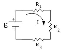
In the above example we want to find a resistor  $R_{eq}$  that is equivalent to  $R_1, R_2, R_3$ .
