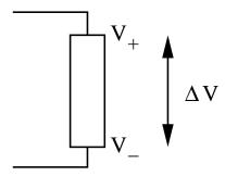
As the charge dq = Idt moves through that potential drop V, it gives up potential energy dV
