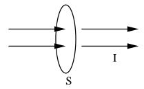
Microscopically, the current density is the product of the amount of charge per unit volume and how fast the charge is moving:
