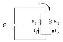
Connected resistances are said to be in parallel when a potential difference that is applied across the combination is the same as the resulting potential difference across the individual resistances. Thus the potential drop across  $R_1$  is the same as that across  $R_2$ :  $\Delta V = I_1 R_1$  and  $\Delta V = I_2 R_2$ .
