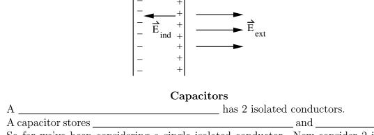
So far we've been considering a single isolated conductor. Now consider 2 isolated conductors. This is a *capacitor*. The conductors are called *capacitor plates*. Capacitors are important circuit elements. They are also used to store energy.
