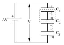
Notice that each capacitor in the series has the same amount of charge on it. To see this, note that the boxed conductor is electrically isolated and therefore has no net charge. The charges are merely separated into +q and -q. No charge can be transferred to the isolated element.
