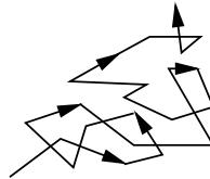
So the drift velocity  $v_d \ll v_e$ . Typically  $v_d \sim 10^{-3}$  m/s. (If you bounce off the walls, it takes longer to get out of the room.)
