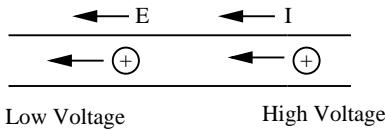
To define current, imagine an imaginary plane passing through a wire like a screen in a pipe. If  $dq$  is the amount of charge passing through the plane in a time  $dt$ , then the current  $I$  is given by
