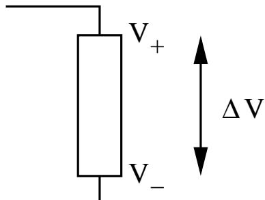
As the charge  $dq = Idt$  moves through that potential drop  $V$ , it gives up potential energy  $dV$
