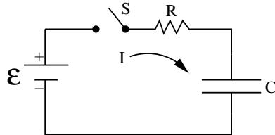
According to the loop rule, we get (using  $q = C\Delta V \implies \Delta V = q/C$ )
