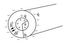
Solution: Assume the inner cylinder has charge +q and  $\sigma_+=q/A_+=q/2\pi aL$ . The outer cylinder has -q and  $\sigma_-=-q/A_-=q/2\pi bL$ .
