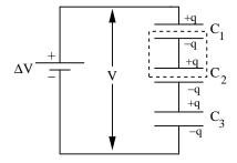
Notice that each capacitor in the series has the same amount of charge on it. To see this, note that the boxed conductor is electrically isolated and therefore has no net charge. The charges are merely separated into +q and -q. No charge can be transferred to the isolated element.
