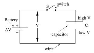
Current starts to flow and the capacitor starts charging once the switch S is closed. Once C is charged, it will stay charged even if S is opened, i.e., +q and -q stay on the plates.
