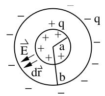
Solution: Assume the inner sphere has charge +q. Find  $\vec{E}$  between the spheres. We know that outside the sphere of charge +q,  $\vec{E}$  is the same as for a point charge:
