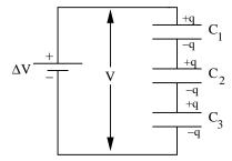
Capacitors are connected in series when the potential difference applied across the combination is the sum of the potential differences across each capacitor.  $C_{eq}$  has the same q and the same  $\Delta V$  as the whole combination.
