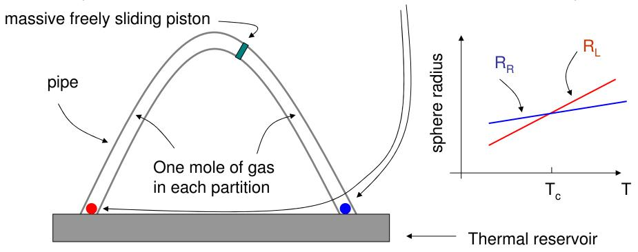
In the absence of spheres and at low enough temperature, the position of the piston at the apex of the pipe is unstable equilibrium due to the gravitational energy cost.
