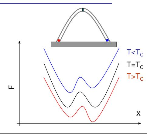
As the temperature of the system is lowered through the transition temperature  $T_c$ , the global energy minimum shifts from right to left. This change is discontinuous, a macroscopic coordinate of the system, x, changes by a discontinuous jump.
