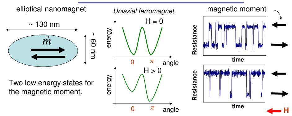
Since the magnet is small enough, fluctuations constantly take the magnet between the states of two opposite directions of magnetic moment.
