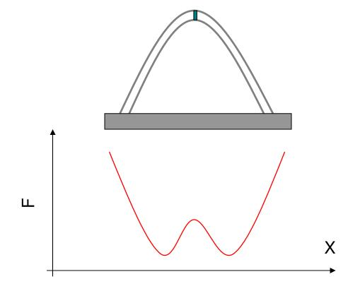
In the presence of spheres and at low enough temperature, the position of the piston at the apex of the pipe is still unstable but the two minima are not equivalent at any temperature other then  $T_c$ .
