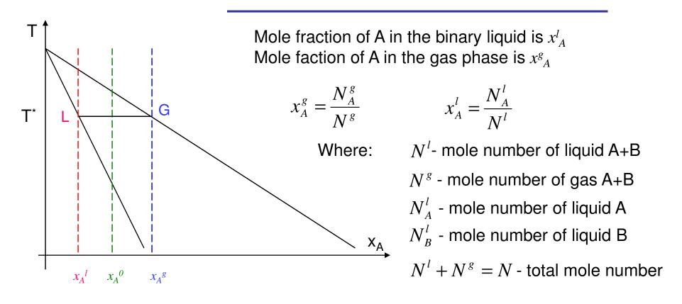
Mole fractions of liquid and gas A are related via the phase diagram on the left:
