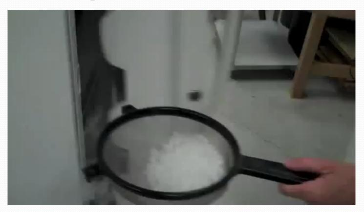
Pour liquid nitrogen to a depth of about 1cm, into lower pan through top sieve to cool both pieces. (You will have to wait while it boils and add more until the temperature stabilizes and the liquid nitrogen remains in the pan)
