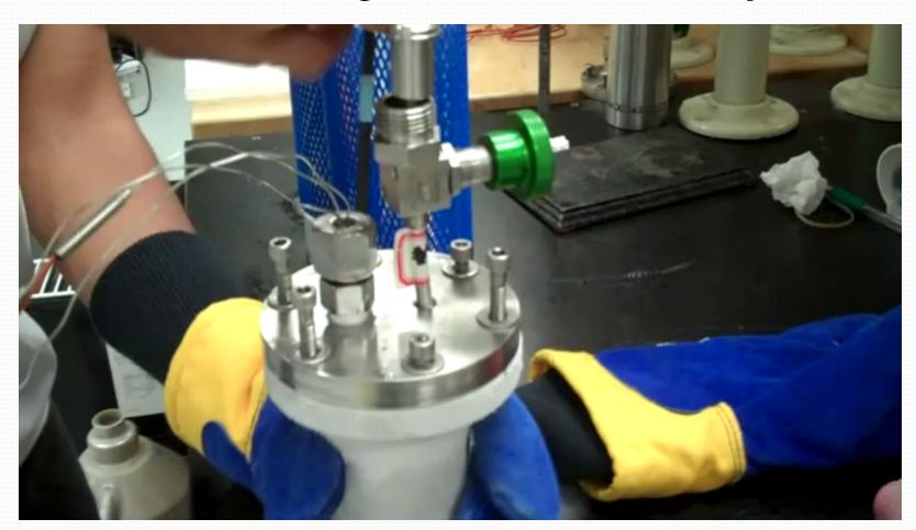
Place pressure cell into ethylene glycol water bath set to a minimum of -3°C and tighten all screws. Make certain pressure valve is closed
