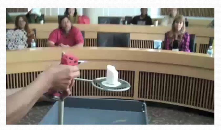
Sample #2 of a propane clathrate hydrate made in the Janda Lab at UCI, July 2010, burning inside a fume hood.
