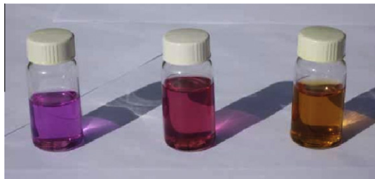
Fig. 1. Iodine in cyclohexane, dichloromethane and water. Why are the colors so different? Could you guess which is which?
