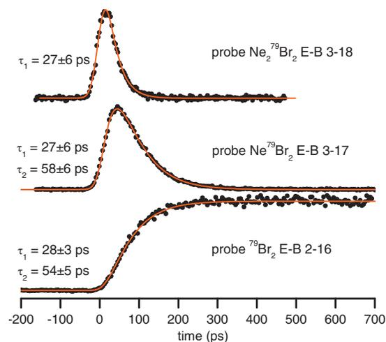
FIG. 7. Delay scans recorded with the pump pulse fixed to excite Ne<sub>2</sub>Br<sub>2</sub> (B, ν' = 18) and the probe pulse fixed to detect the initial Ne<sub>2</sub>Br<sub>2</sub> (B, ν' = 18), intermediate NeBr<sub>2</sub> (B, ν' = 17), and product Br<sub>2</sub> (B, ν' = 16). The red curve shows the fit to the data assuming a sequential first order kinetic mechanism. The time constants listed are those extracted from the fitting procedure.
