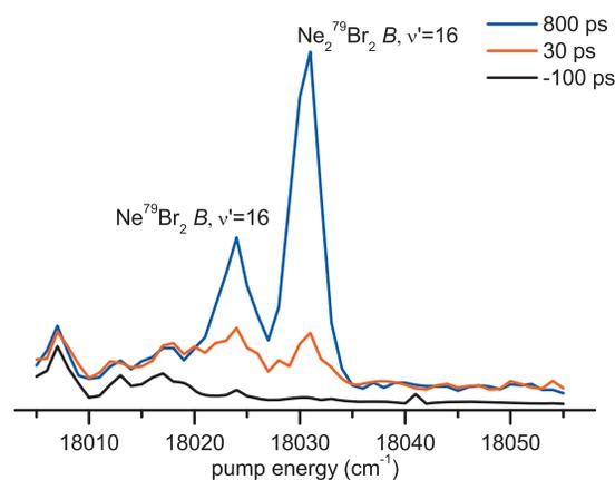
FIG. 2. Excitation spectra over the  $B \leftarrow X$ ,  $16 \leftarrow 0$  region obtained with the probe laser fixed on the  $\text{Br}_2$   $E \leftarrow B$ ,  $1 \leftarrow 14$  transition. The spectra were taken with the probe delayed relative to the pump by  $-100$  ps (black), 30 ps (red), and 800 ps (blue).
