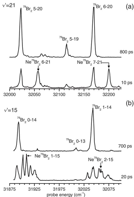
FIG. 4. Probe spectra recorded with the pump pulse fixed to excite (a) NeBr<sub>2</sub> ( $B, \nu'=21$ ) and (b) NeBr<sub>2</sub> ( $B, \nu'=15$ ). The labels on the peaks denote the  $E \leftarrow B, \nu \leftarrow \nu'$  vibronic transitions. Each spectrum is labeled on the right according to the time delay of the probe relative to the pump.
