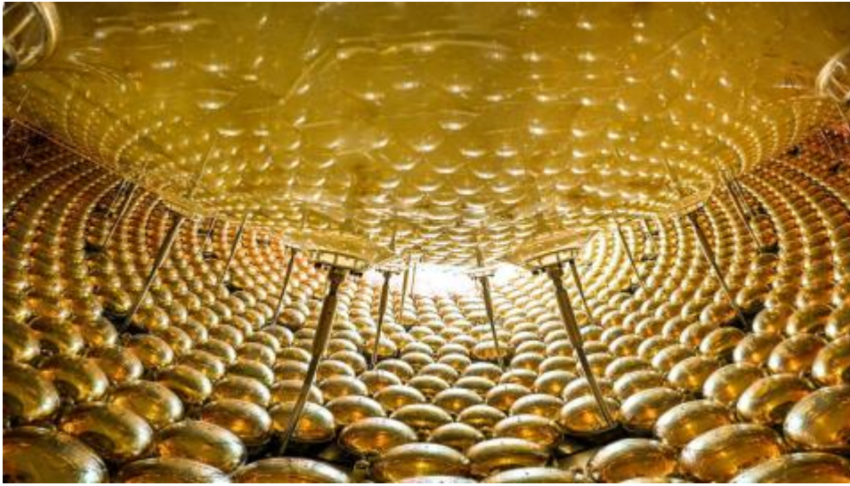
JUNO's golden photomultiplier tubes line the inside of the detector. These extremely sensitive semispheres detect the light produced by neutrino interactions. Yuexiang Liu / Institute of High Energy Physics
