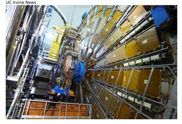
At CERN's Large Hadron Collider, technicians install the New Small Wheels upgrade at the ATLAS experiment; it's designed to help trigger and track elementary particles known as muons. UC Irvine researchers led the commissioning of NSW and were among a large group of scientists to win this year's Breakthrough Prize in Fundamental Physics.
