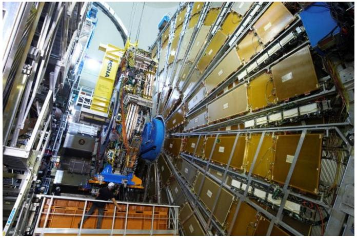
At CERN's Large Hadron Collider, technicians install the New Small Wheels upgrade at the ATLAS experiment; it's designed to help trigger and track elementary particles known as muons. UC Irvine researchers led the commissioning of NSW and were among a large group of scientists to win this year's Breakthrough Prize in Fundamental Physics. Picture Credit: Julien Marius Ordan / CERN
