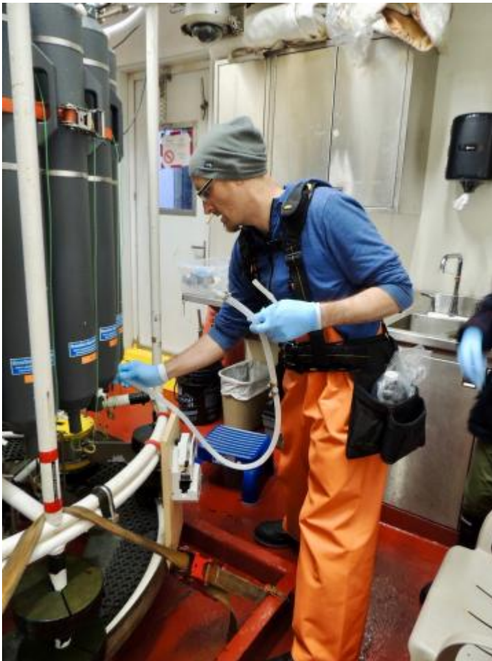
Brett Walker, associate professor of Earth system science, samples Baffin Bay seawater from the CTD (conductivity, temperature, depth) Rosette equipped with depth-specific sampling bottles. Sara Zeidan / University of Ottawa
