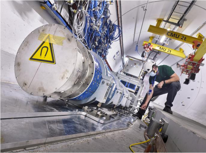
The FASER particle detector, located deep underground at CERN's Large Hadron Collider, was mostly built out of spare parts from other experiments at CERN. Photo courtesy of CERN.
