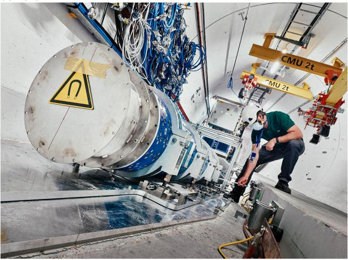
The FASER particle detector that received CERN approval to be installed at the Large Hadron Collider in 2019 has recently been augmented with an instrument to detect neutrinos. The UCI-led FASER team used a smaller detector of the same type in 2018
