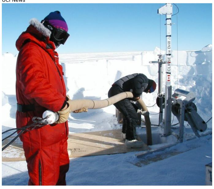
Researchers insert a vacuum line down a borehole in Megadunes, Antarctica, to pump air out of the snow pack. Researchers at UCI analyzed the "firn" air to determine that the amount of molecular hydrogen in Earth's atmosphere has increased by 70 percent since the mid 1800s.
