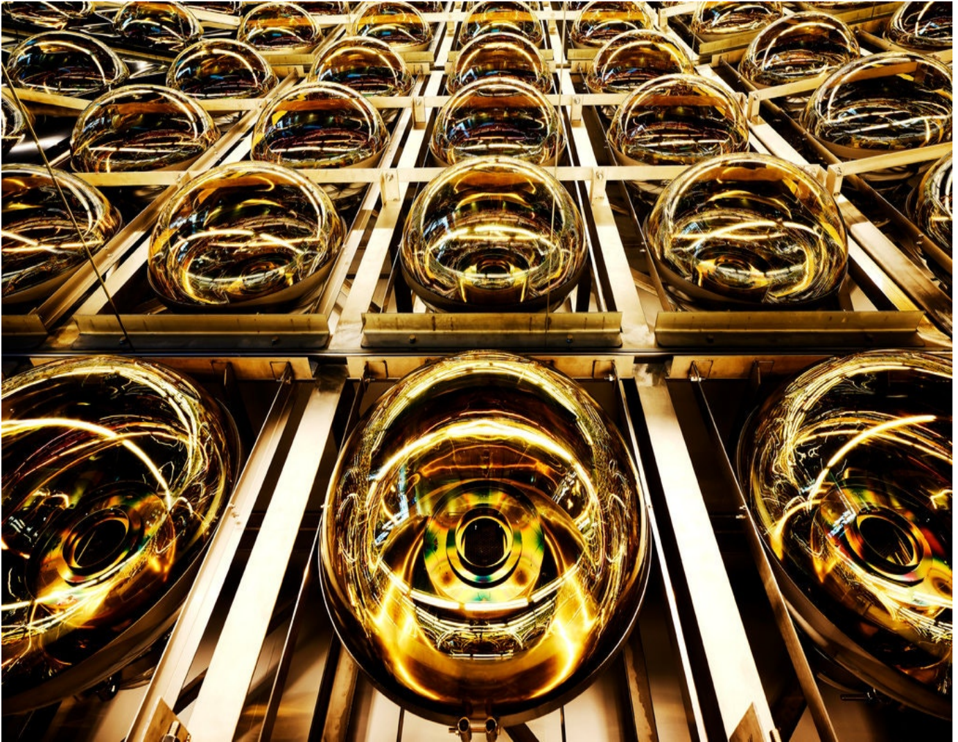
A mock-up of the more than 13,000 photomultiplier tubes inside the Super-Kamiokande neutrino detector. Credit... Enrico Sacchetti/Science Source
