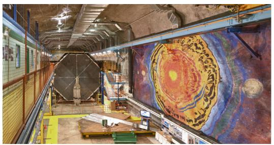
For the MINOS+ experiment, Fermilab accelerators send a beam of muon neutrinos through a detector located on the Fermilab site. The beam traveles 450 miles underground to a far detector, pictured here, in northern Minnesota. Reidar Hahn, Fermilab
