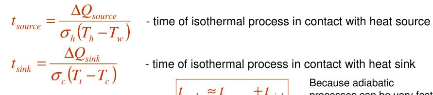
$t_{cycle} \approx t_{source} + t_{sink}$  Because adiabatic processes can be very fast
